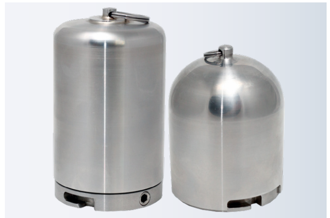
BCA 500 EX and DC bombs for low and high pressure combustion respectively
